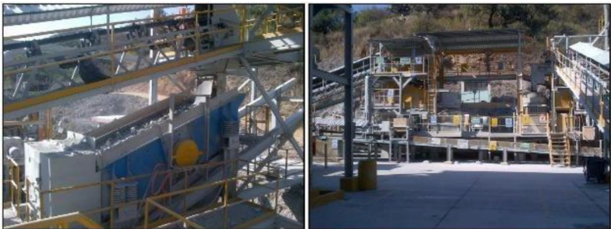
Figure 17-4 Vibration Screen, Single 6'x16'Deck (left); Fine Crushing Circuit (right)
