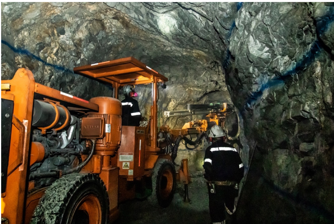
A Jumbo Drill working to provide access to additional stopes at El Cubo
